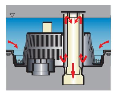
The original MEIKO eco filter system in all EcoStar diswashers allows for an optimal wash water filtering - this means that clean tank water can be used longer and more efficiently and that outstanding hygienic cleaning results are achieved.
